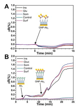
Fig. 5 Real-time SPR angle shift sensorgrams of (A) the nonspecific binding effect of GNP-Ab2 conjugates and (B) the specific binding effect of GNP-Ab<sub>2</sub> conjugates after primary antibody injection (blank injection C<sub>0</sub>). Immobilized BSA and the bare SAM surface identified as "Control" and "Surf" were used as negative controls.
