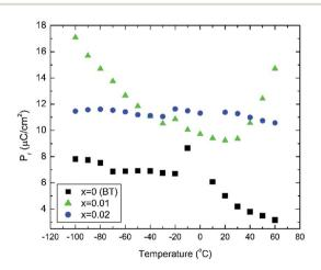
Fig. 3 Temperature dependence of the remanent polarisation,  $P_r$ , for (1-x)BaTiO<sub>3</sub>-xBiYbO<sub>3</sub> ceramics.
