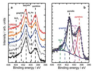
Fig. 2 (a) High resolution N 1s XPS data of PANI samples with different N precursors. (b) Example of the deconvolution of a N 1s spectrum acquired for the MEL sample.
