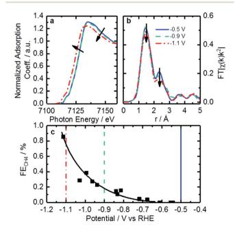
Fig. 7 Fe K-edge XANES (a) and EXAFS (b) spectra taken under *operando* conditions in  $CO_2$ -saturated 0.1 M KHCO $_3$  at -0.5 V (solid blue curves), -0.9 V (dashed green curves) and -1.1 V (red dot-dashed curves) vs. RHE. (c) Faradaic efficiency to  $CH_4$  varying with potential. Lines are added to indicate points representative of spectra in (a) and (b).
