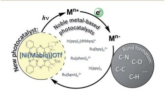
Scheme 1 Photoredox catalysis commonly relies on noble metal complexes for organic transformations, initiated by single electron transfer upon excitation of Ru or Ir compounds. The [Ni(Mabiq)]OTf catalyst offers an earth-abundant photosensitizer.
