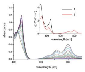
Fig. 2 Spectral evolution during photoconversion of 1 to 2 [c (1) = 0.05 mM; c (NEt<sub>3</sub>) = 1.4 M;  $\lambda$  = 457 nm, DMF]. Inset: electronic spectra of 1 (black trace; CH<sub>2</sub>Cl<sub>2</sub>) and 2 (red trace; THF).
