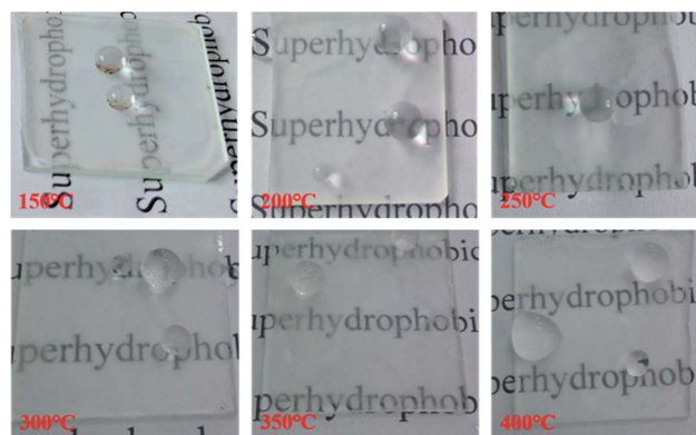
Fig. 8 Optical images of water droplets on the glass coated by the P-MSA-I/Qsil 216 composite after high temperature calcination for 4 h.
