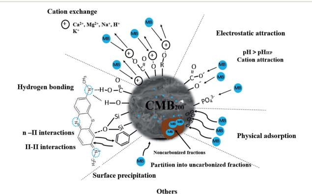
Fig. 10 Interaction mechanisms in the biochar-MB system.
