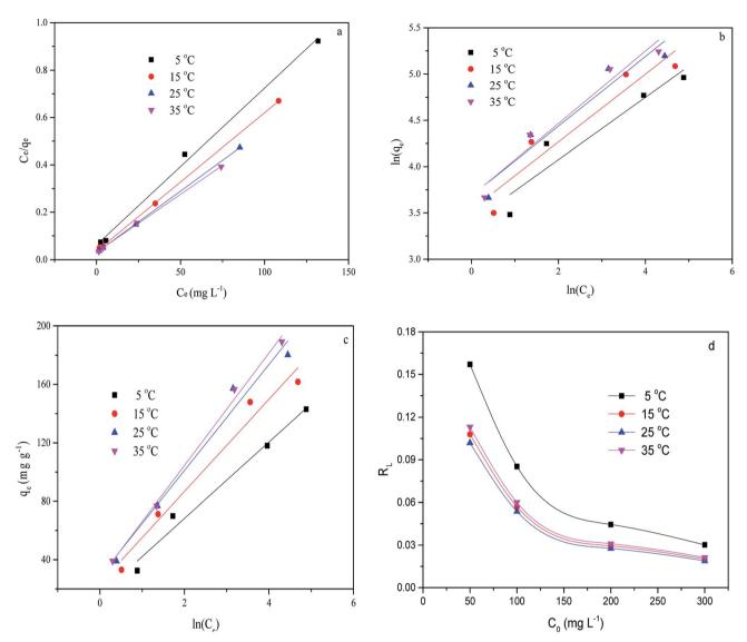
Linear fits of the adsorption of MB on CMB predicted by various isotherm models. (a) Langmuir; (b) Freundlich; (c) Temkin; (d)  $R_L$
