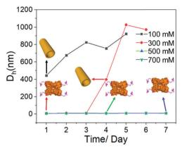
Fig. 5 Time-dependent DLS results of SBA/R3GN with different concentrations (100 mM, 300 mM, 500 mM and 700 mM) of Ca(NO<sub>3</sub>)<sub>2</sub> at 4 °C (pH = 6.0, [SBA]: 0.1 mM and [R3GN]: 0.2 mM). The inset cartons correspond to the mixture state of SBA/R3GN at different incubation times and concentrations of Ca(NO<sub>3</sub>)<sub>2</sub> at 4 °C.
