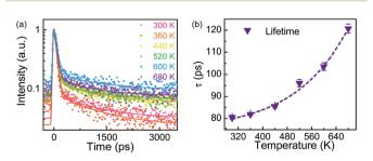
Fig. 5 (a) Time-resolved PL spectra of the  $K \rightarrow K$  direct emission at different temperatures. The solid lines are exponential decay fittings of the obtained experimental data points, giving out the effective fluorescence lifetime of the  $K \to K$  direct emission. (b) The fitted effective lifetime  $\tau$  as a function of the measurement temperature
