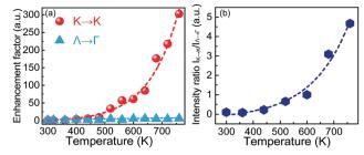
Fig. 4 (a) Enhancement factor of the  $K \to K$  direct and  $\Lambda \to \Gamma$  indirect emissions at different temperatures. (b) Temperature dependence of the integrated intensity ratio of the  $K \to K$  direct emission to the  $\Lambda \to \Gamma$  indirect emission  $(I_{K \to K}/I_{A \to \Gamma})$ .
