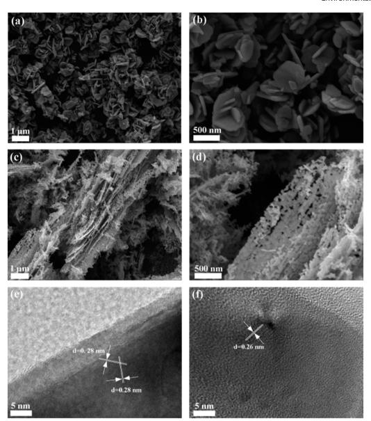
Fig. 2 SEM images of ZnO nanomaterials: ZnO-0001 with (a) low and (b) high magnification, ZnO-1010 with (c) low and (d) high magnification. HRTEM images of (e) ZnO-0001 and (f) ZnO-1010.
