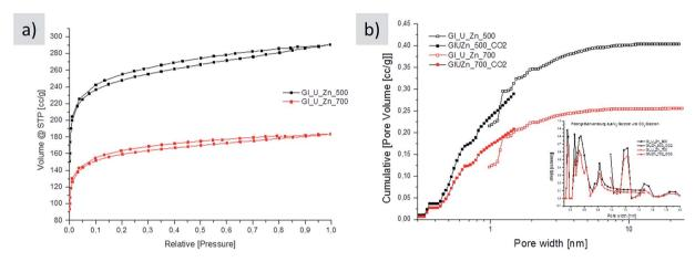
Fig. 3 (a) Nitrogen sorption isotherms and (b) pores size distribution from nitrogen (open circles) and CO<sub>2</sub> (filled circles) sorption of carbons made from glucose, urea, and ZnCl<sub>2</sub> carbonized at 500 °C (black) and 700 °C (red).
