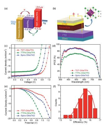
Fig. 4 (a) Energy level diagram for each layer of the PSC device based on the TDT-OMeTPA HTM. (b) Schematic of the planar PSC device. (c) J-V curves under simulated 1.0 M sunlight, (d) IPCE curves, and (e) J-V curves in the dark of PSC devices based on TDT-OMeTPA, TTPA-OMeTPA and Spiro-OMeTAD. (f) Histogram of 30 device PCEs based on the TDT-OMeTPA HTM.
