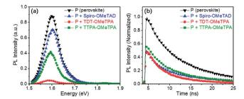
Fig. 6 (a) The time-integrated photoluminescence spectra of the perovskite films with/without the different HTMs. (b) The timeresolved photoluminescence spectra measured at a wavelength near the band gap that yields the maximum photoluminescence signal upon exciting the perovskite films containing the different HTMs at 420 nm
