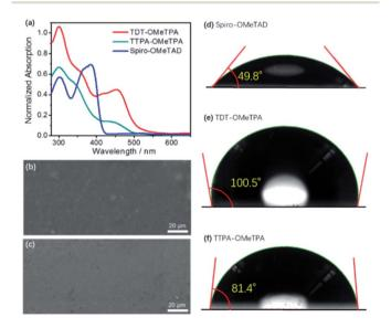
Fig. 2 (a) UV-vis absorbance of TDT-OMeTPA, TTPA-OMeTPA and Spiro-OMeTAD. SEM images of the (b) TDT-OMeTPA and (c) TTPA-OMeTPA layers accumulated on perovskite layers. Water contact angles on (d) Spiro-OMeTAD, (e) TDT-OMeTPA and (f) TTPA-OMeTPA.
