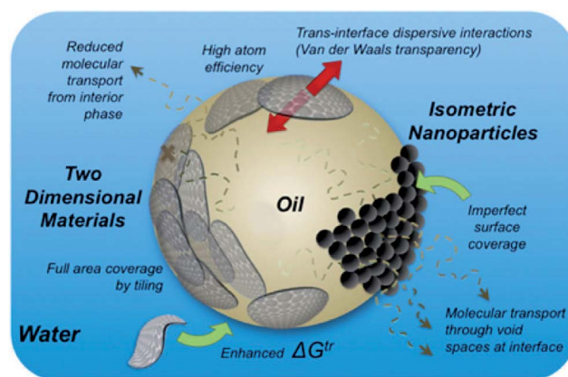
Fig. 5 Schematic illustrates advantage of two-dimensional nanosheets over zero-dimensional nanoparticles to stabilize emulsions. (Reprinted with permission from (ref. 60). Copyright (2014) American Chemical Society.)
