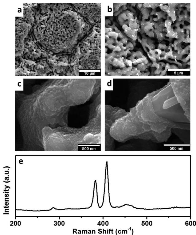
Fig. 3 (a–c) Scanning electron micrographs of  $\text{MoS}_2$  covered 3D stainless steel-graphene structures. A highly conformal coating on the surface is achieved by electrodeposition technique. The porous nature of the current collector is preserved with no clogging or large particulates; (d) an isolated defect in the electrodeposition, shown to highlight the thickness of the  $\text{MoS}_2$  layer; (e) Raman spectrum of the structure wherein the bands correspond to  $\text{MoS}_2$ .
