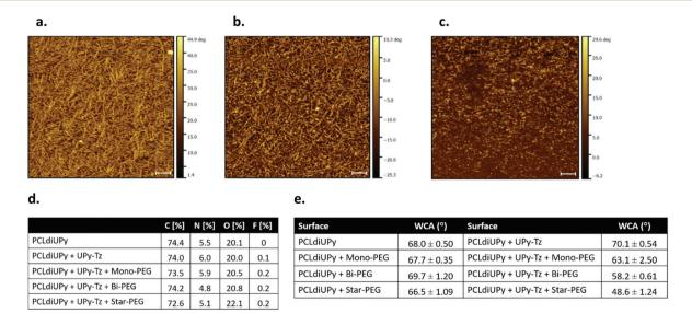
Fig. 2 Surface characterization of the different material films with AFM, XPS and water contact angle. AFM phase micrographs of PCLdiUPy (a), PCLdiUPy with 10 mol% UPy-Tz (b) and after star-PEG-BCN functionalization (c), (d) XPS compositional table of the different surfaces and (e) water contact angles of the respective surfaces. Five measurements were performed per surface and standard deviations are plotted.
