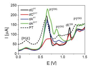
**Fig. 8** Comparison of SWV responses of PTZ and PT- or EPT-modified nucleosides. SWV parameters: frequency 200 Hz, amplitude 50 mV,  $E_{\rm i}$  = 0.0 V. Peak denoted as (PGE) is produced by the electrode due to the presence of oxygenous functional groups at its surface. For other details, see Fig. 7.
