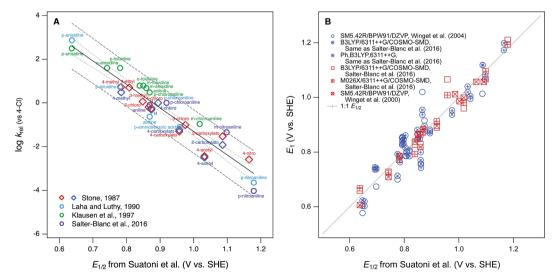
Fig. 1 Examples of correlation analyses performed using  $E_{1/2}$  for phenols and anilines from Suatoni *et al.* as the descriptor variable. (A) Rate constants ( $k_{rel}$ ) for oxidation by manganese oxides; (B) one-electron oxidation potentials ( $E_1$ ) calculated from theory. In (A), diamonds represent phenols and circles represent anilines.
