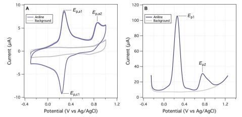
Fig. 2 Electrochemical data from this study, using aniline as an example. (A) Staircase cyclic voltammetry (SCV) at a scan rate of 125 mV s<sup>-1</sup> and (B) square-wave voltammetry (SWV) at a scan rate of 60 mV s<sup>-1</sup> and amplitude of 75 mV. Both for 0.25 mM aniline in 25% IPA/buffer, pH<sub>meas</sub> 5.1 and step size 2 mV
