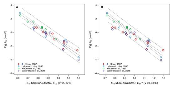
Fig. 6 Correlations of rate constants for oxidation by manganese oxides ( $k_{rel}$ ) and oxidation potentials of phenols and anilines: (A) log  $k_{rel}$  from compiled sources (Table S1†) vs.  $E_1$  with calibration using data for  $E_{1/2}$ ; (B)  $\log k_{\rm rel}$  from compiled sources vs.  $E_1$  with calibration using data for  $E_{\rm pl}^{\rm 1st}$  (Tables S9 and S10†). Diamonds represent phenols and circles represent anilines.
