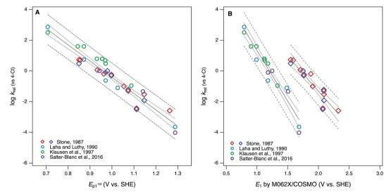
Fig. 5 Correlations of rate constants for oxidation by manganese oxides ( $k_{rel}$ ) and oxidation potentials of phenols and anilines: (A) log  $k_{rel}$  from compiled sources (Table S1†) vs.  $E_{D1}^{1st}$  from this study (Tables S4 and S5†); (B) log  $k_{rel}$  vs.  $E_1$  without calibration, from this study (Tables S6 and S7†). Diamonds represent phenols and circles represent anilines.
