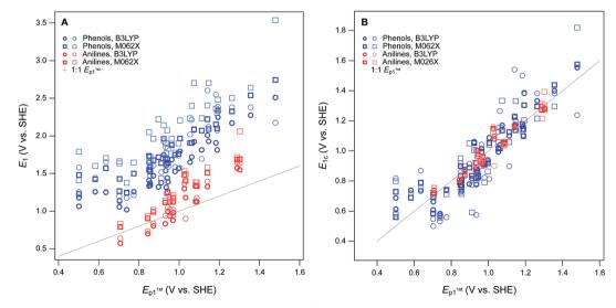
Fig. 4 Comparisons between measured  $E_1$  (without calibration) and  $E_{\text{p1}}^{\text{lst}}$  for phenols and anilines. (A) Direct comparison between measured potentials, (B) statistical analysis of the calibration equations from regression of  $E_1$  and  $E_{11}^{\rm st}$  (shown in Fig. S6†). In (A) and (B), phenols and anilines are distinguished, not combined.
