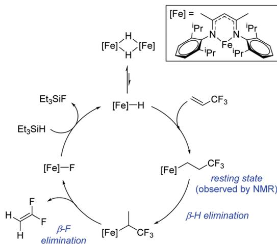
**Scheme 8** Postulated catalytic cycle for hydrodefluorination of fluoroolefins.
