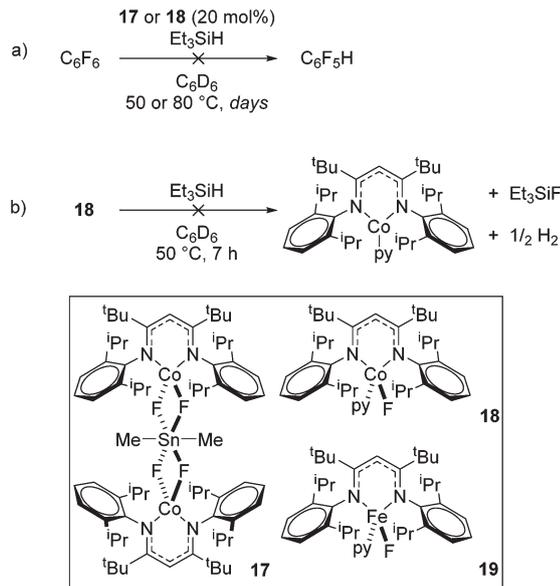
**Scheme 17** (a) Hydrodefluorination is not catalytic with respect to cobalt. (b) Stoichiometric reaction with silanes does not produce Co-hydride, which is expected to be a reactive intermediate in a successful hydrodefluorination catalytic cycle.
