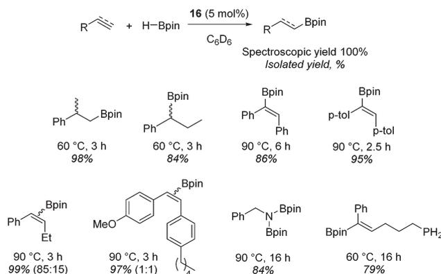
**Scheme 16** Alkene and alkyne hydroboration can be carried out with **15**, however, a vast improvement in reactivity is observed with **16** and this allows the hydroboration of challenging substrates.
