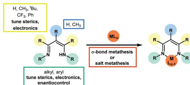
**Scheme 1** The utility of the  $\beta$ -diketiminato ligand stems from the steric and electronic parameters that can be readily tuned, whilst the varied methods available to introduce the metal centre and co-ligands is synthetically advantageous.
