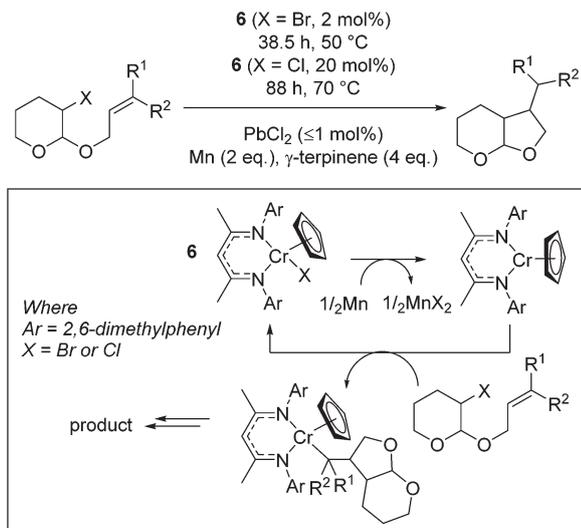
**Scheme 6** Halo-acetals form furo-pyran structures using Cr–Cp catalyst **6**. The chemistry can be applied to both bromo- and chloro substrates, with the bromo-acetal undergoing conversion to product more rapidly and at lower temperature.
