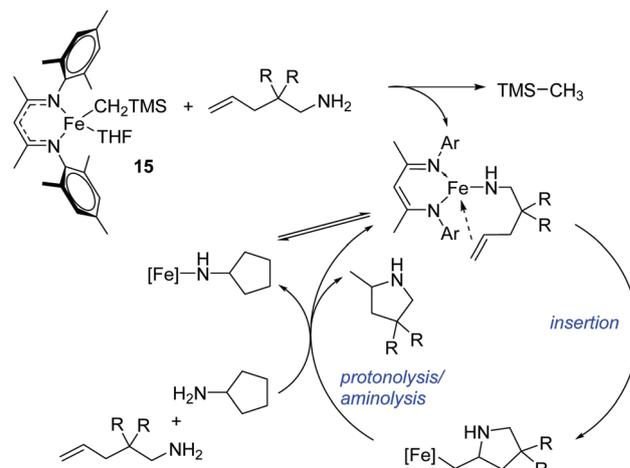
**Scheme 11** Hannedouche's postulated mechanism for intramolecular hydroamination.
