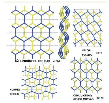
Fig. 9 The four patterns of entanglement observed in 2-fold interpenetrated hcb. The HRNs are represented by dotted lines. The undulation of the layers for the most common pattern ERN (3,6)II is shown from the lateral views. B11a-c refer to the corresponding figures in ref. 3. See also Scheme 2.
