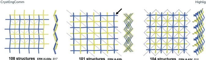
Fig. 8 The three most common patterns of entanglement observed in 2-fold interpenetrated sql. The HRNs are represented by dotted lines. The undulation and bending of ligands is visible from the lateral views. B17 and B18 refer to the corresponding figures in ref. 3. See also Scheme 1.
