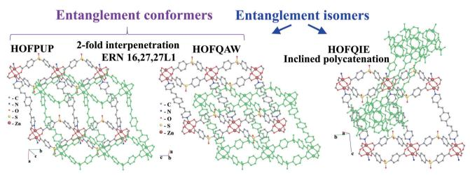
Fig. 13 Networks of interpenetrating conformers (left) [Zn<sub>2</sub>(pdedp)(sdb)<sub>2</sub>]·2DMA·2H<sub>2</sub>O (HOFPUP) and [Zn<sub>2</sub>(pdedp)(sdb)<sub>2</sub>]·Me<sub>2</sub>SO (HOFQAW) with 2-loops catenation and (right) the inclined polycatenated isomer [Zn<sub>2</sub>(pdedp)(sdb)<sub>2</sub>]·DMF·Me<sub>2</sub>SO·1.5H<sub>2</sub>O (HOFQIE) without 2-loops catenation.
