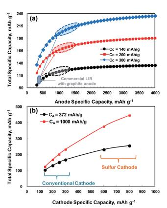
Fig. 1 Total specific capacity of a LIB cell as a function of the specific capacity of (a) anode and (b) cathode.
