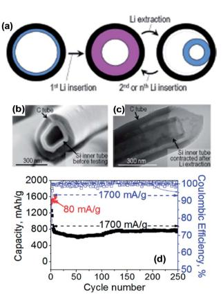
Fig. 5 (a) Results of the computational modeling of shape changes of a Si tube inside a rigid nanopore during reaction with Li, (b) SEM image of the composite Si-in-C tubes, (c) TEM image after Li extraction at the 10<sup>th</sup> cycle, and (d) deintercalation capacity retention and coulombic efficiency for the sample containing 33 wt% Si. The reported capacity is normalized by the total weight of C and Si. Reproduced with permission.61 Copyright 2010, American Chemical Society.
