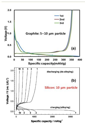
**Fig. 2** Typical galvanostatic charge–discharge voltage profiles obtained with anodes of (a) graphite powder and (b) silicon powder having sizes on the order of micrometers. (b) is reproduced with permission.<sup>48</sup> Copyright 2004, The Electrochemical Society.
