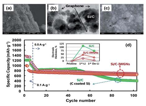
Fig. 10 (a) SEM and (b) TEM images of a Si/C-IWGN composite, and (c) SEM image of a particle cross-section of a Si/C-IWGN composite, and (d) cycling performances of Si/C and Si/C-IWGN composites (the inset shows electrode thickness increases of Si/C and Si/C-IWGNs electrodes during the 1st charge-discharge cycles). Reproduced with permission. Copyright 2015, Royal Society of Chemistry.
