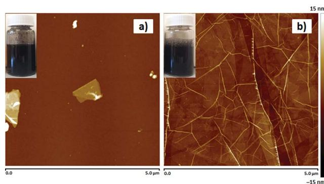
Fig. 1 AFM images ( $5 \times 5\ \mu\text{m}^2$ ) of chemically reduced graphene oxide (CRGO) (a) without and (b) with SDBS. Insets show digital photographs of the corresponding samples in an aqueous  $1\ \text{mg mL}^{-1}$  solution.
