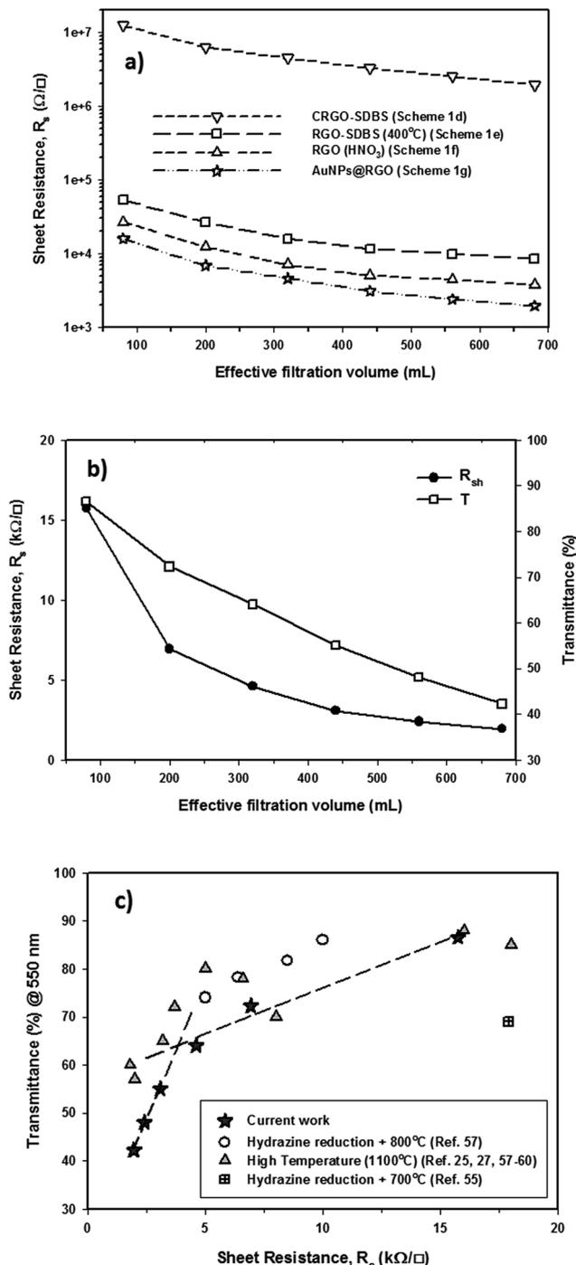
Fig. 4 (a)  $R_s$  vs. thickness of the graphene films prepared from four different structures; (b)  $R_s$  and transmittance (at  $\lambda = 550$  nm) of selected TCGFs with different thicknesses; (c) comparison of  $R_s$  as a function of transmittance (at  $\lambda = 550$  nm) between our AuNPs-RGO films and other studies. Dash lines show the two regions of differing resistance for the graphene films and the threshold transmittance and corresponding  $R_s$ .
