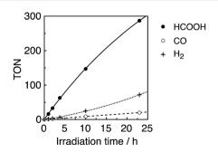
Fig. 8 Photocatalytic CO<sub>2</sub> reduction using R(5) (0.05 mM) as the PS and Ru(tBu)-Cl<sub>2</sub> (0.05 mM) as the catalyst in DMA-TEOA (5:1 v/v) under 436 nm light irradiation of  $4.2 \times 10^{-9}$  einstein per s intensity.
