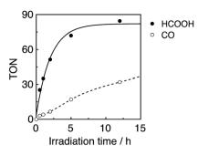
Fig. 10 Photocatalytic CO $_2$  reduction using R(5) (0.05 mM) as the PS and Mn(tBu)-ACN (0.05 mM) as the catalyst in DMA-TEOA (5 : 1 v/v) under 436 nm light irradiation of 5.3  $\times$  10<sup>-9</sup> einstein per s intensity.
