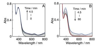
Fig. 11 UV-vis absorption spectral changes of a CO<sub>2</sub>-saturated DMA–TEOA (5:1 v/v) solution containing R(5) (0.05 mM) as the PS and Mn(tBu)-ACN (0.05 mM) as the catalyst, under irradiation at  $\lambda_{\rm ex}=436$  nm (5.3  $\times$  10<sup>-9</sup> einstein per s) in the initial stage (A) and over 1 h irradiation (B).
