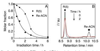
Fig. 6 (A) Residual R(5) and Re-ACN in solution during the photocatalytic reaction, obtained using UPLC analysis (Fig. S9, ESI†). (B) UPLC chart of the photocatalytic system R(5)/Re-ACN before and after 2 h of irradiation;  $\lambda_{\text{det}} = 350$  nm.
