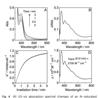
DMF-TEOA (5 : 1 v/v) solution containing R(5) (0.05 mM) under irradiation at  $\lambda_{\rm ex}=436$  nm (5.6  $\times$  10<sup>-9</sup> einstein per s). (B) Differential absorption spectrum before irradiation and after 3 min irradiation. (C) Time course of accumulated electrons in R(5), compensated for the inner filter effect. (D) Differential absorption spectrum of R(5) before and after bulk electrolysis in an Ar-saturated DMF solution at -1.95 V vs. Ag/AgNO<sub>3</sub>.
