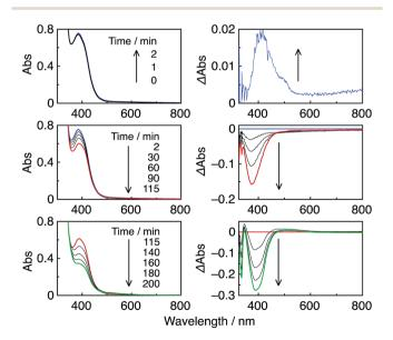
Fig. 5 UV-vis (left) and the corresponding differential absorption spectral changes (right) during the irradiation of a CO2-saturated DMF-TEOA (5:1 v/v) solution containing R(5) (0.05 mM) as a PS and Re-ACN (0.05 mM) as the catalyst, under irradiation at  $\lambda_{ex} = 436$  nm  $(5.7 \times 10^{-9} \text{ einstein per s})$  in the initial stage (top) and over 3.5 h irradiation (middle and bottom).
