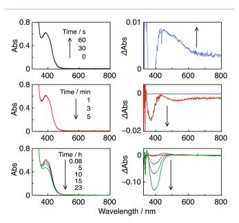
Fig. 9 UV-vis (left) and the corresponding differential absorption spectral changes (right) during the irradiation of a CO<sub>2</sub>-saturated DMA–TEOA (5 : 1 v/v) solution containing R(5) (0.05 mM) as the PS and Ru(tBu)-Cl<sub>2</sub> (0.05 mM) as the catalyst, under irradiation at  $\lambda_{\rm ex}=436$  nm  $(4.2\times10^{-9}$  einstein per s).
