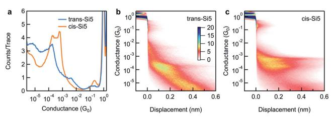
Fig. 3 (a) Logarithmically binned one-dimensional conductance histogram of cis-Si5 (orange) and trans-Si5 (blue). Histograms are made without data selection and normalized by the total number of traces. (b) and (c) Two-dimensional conductance histograms of trans-Si5 and cis-Si5 respectively, made from the same data as in (a).
