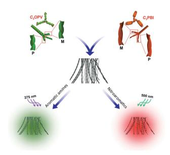
Fig. 9 Schematic illustration of the fluorescence 'turn-off/turn-on' mechanism of the self-sorted fibres of a 1:1 mixture of  $C_3$ OPV and  $C_3$ PBI on exposure to different VOCs.
