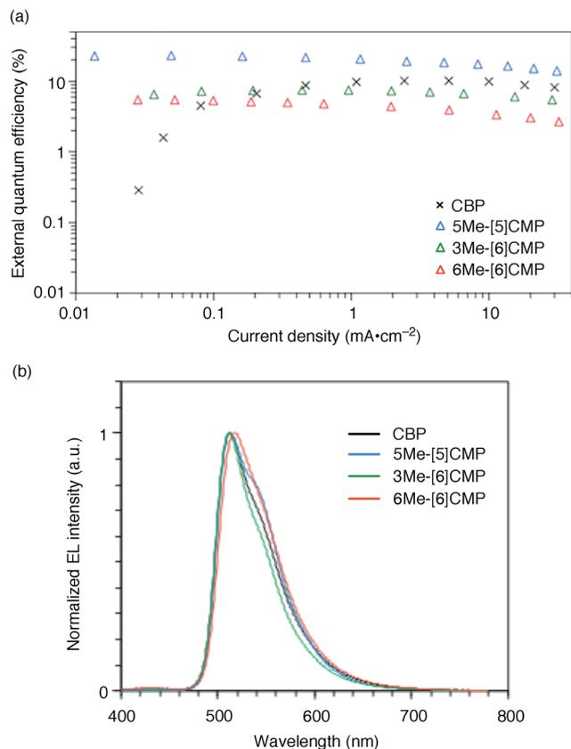
Fig. 5 Performance of the single-layer OLED. (a) External quantum efficiency of the single-layer OLED plotted against the current density. See Fig. 1a for the device architecture. (b) Electroluminescence spectra at a current density of  $0.1 \text{ mA cm}^{-2}$ .
