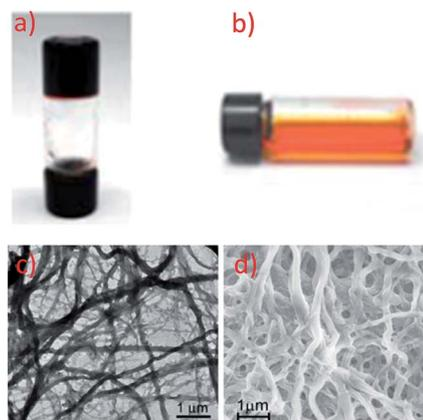
Fig. 11 Photographs of **67** in DMSO in (a) the gel form at room temperature, (b) the sol form at elevated temperature. (c) TEM and (d) SEM images of the xerogel of **67** formed in DMSO (adapted from ref. 118 with permission from the Royal Society of Chemistry).
