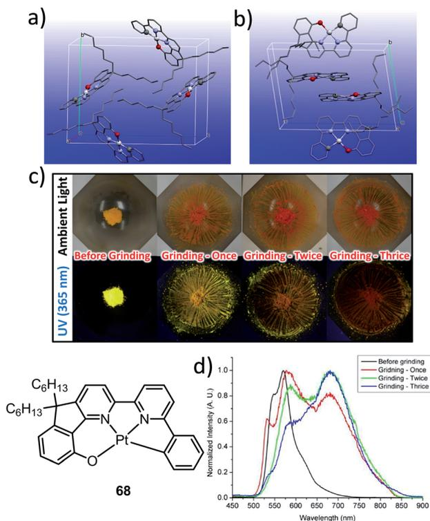
Fig. 12 Crystal packing of **68** in (a) monoclinic form and (b) triclinic form. (c) Photographs of the yellow crystalline solid of **68** before and after grinding under ambient and UV light irradiation (365 nm). (d) Emission spectra of **68** (yellow triclinic form) before and after grinding.
