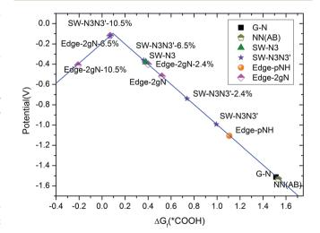
Fig. 7 Calculated limiting potentials for  $CO_2$  to CO reduction. Curvature is added by reducing the lattice parameter along the X direction (shown in Fig. 2), which is presented by the percentage of lattice parameter reduced.
