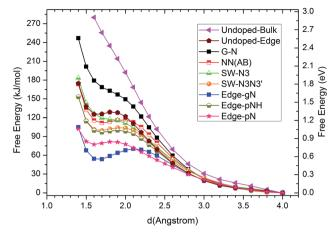
Fig. 3 Free energy profiles of CO<sub>2</sub> approaching C sites with large DOS just below the Fermi level in N doped graphenes for G-N, NN(AB), SW-N3, SW-N3N3', Edge-gN, Edge-pN, Edge-pNH and un-doped bulk surface and edge structures. The approaching distance is that between C atom in CO<sub>2</sub> and the candidate sites in catalysts. The free energy profile for O atom in CO2 approaching candidate sites are also checked in ESI.†
