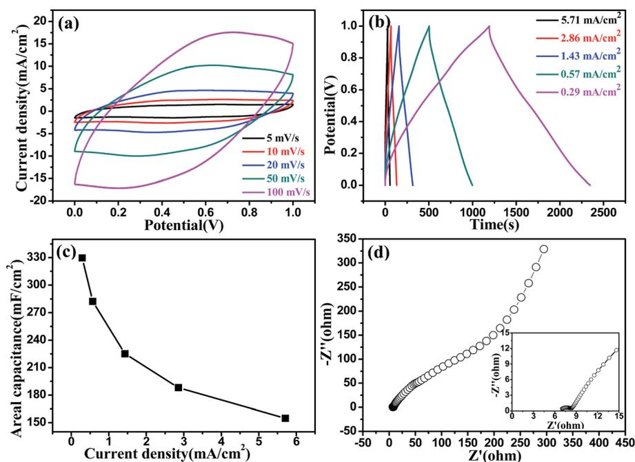
Fig. 2 (a) CV curves of the helical  $\text{Na}_x\text{MnO}_2$  at different scan rates; (b) GCD curves of the helical  $\text{Na}_x\text{MnO}_2$  at different current densities in 1.0 M  $\text{Na}_2\text{SO}_4$  electrolyte; (c) areal capacitance calculated from GCD curves as a function of current densities; (d) EIS spectra of the  $\text{Na}_x\text{MnO}_2$  (inset is the enlarged view of the high frequency region).
