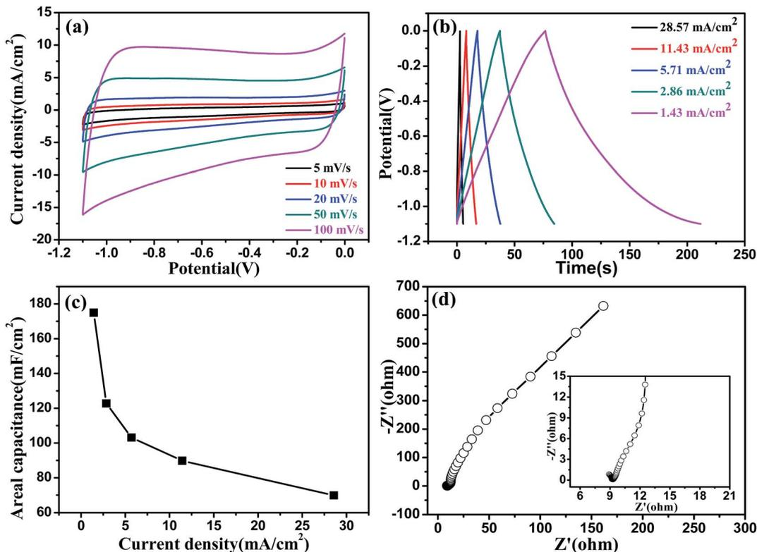
Fig. 4 (a) CV curves at different scan rates; (b) GCD curves at different current densities of the helical  $\text{MoO}_2$  in 1.0 M  $\text{Na}_2\text{SO}_4$  electrolyte; (c) areal capacitance calculated from GCD curves as a function of current densities; (d) EIS spectra of  $\text{MoO}_2$  (inset is the enlarged view of the high frequency region).
