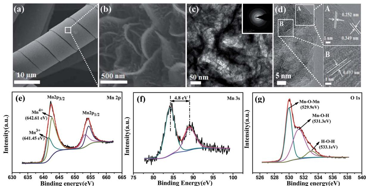
Fig. 1 (a and b) SEM images of the helical  $\text{Na}_x\text{MnO}_2$  with hierarchical porous structures; (c) TEM and (d) HRTEM images of the typical  $\text{Na}_x\text{MnO}_2$  nanosheets (inset in (c) is the SAED pattern); XPS spectra of the helical  $\text{Na}_x\text{MnO}_2$  of (e) Mn 2p, (f) Mn 3s, and (g) O 1s.
