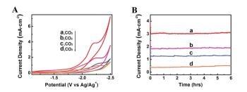
Fig. 6 CV traces (A) and current density profiles at an applied potential of -2.2 V vs.  $\text{Ag/Ag}^+$  (B) using different kinds of ILs as electrolytes: (a)  $\text{BmimBF}_4$ ; (b) BmimOTf; (c)  $\text{BmimPF}_6$ ; (d)  $\text{BmimClO}_4$ .
