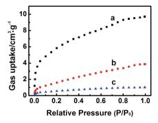
Fig. 8 The adsorption curves of  $\rm CO_2$  (a),  $\rm CO$  (b) and  $\rm CH_4$  (c) at 298 K on the Zn-MOF synthesized at x=0.38.
