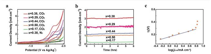
Fig. 4  $CO_2$  reduction performance of Zn-MOF/CP cathodes. (a) CV traces. (b) Current density profiles. (c) Tafel plot for CH<sub>4</sub> of the Zn-MOF/CP cathode using Zn-MOF synthesized at x=0.38.
