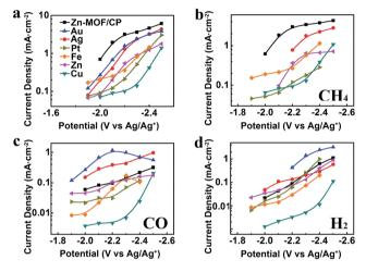
Fig. 7 Current densities obtained from of the Zn-MOF/CP cathode prepared using Zn-MOF synthesized at x=0.38 and various metal cathodes. (a) Total current densities. (b) Partial current densities of CH<sub>4</sub>. (c) Partial current densities of CO. (d) Partial current densities of H<sub>2</sub>.
