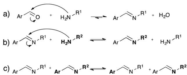
Fig. 10 Reversible processes associated with imine chemistry. (a) Equilibrium of imine formation, *via* intermediate hemi-aminal formation; (b) transamination between imines and amines *via* intermediate aminal formation; (c) imine metathesis.
