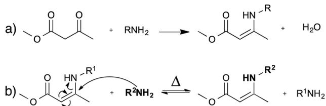
Fig. 5 (a) Synthesis of vinylogous urethane; this reaction can even be performed in water. (b) Exchange of vinylogous urethanes and amines occurs at temperatures above 100 °C without catalyst *via* a Michael addition.
