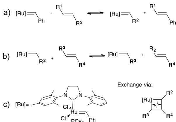
Fig. 8 Olefin metathesis exchange reaction, (a) insertion of the Grubbs' second generation catalyst into an alkyl chain (b) exchange of two alkene bonds (c) left: structure of 2<sup>nd</sup> generation Grubbs' catalyst; right: the associative exchange mechanism of a metathesis reaction.
