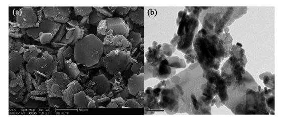
Fig. 3 SEM images (a) and TEM images (b) of Zn-Al LDH (image (a) adapted from ref. 35 with Copyright from 2014 Elsevier and image (b) adapted form ref. 44 with copyright from 2016 Elsevier).
