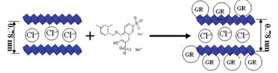
Fig. 10 The models illustration of MO and GR interacted with Ca-Al LDH (adapted from ref. 119 with copyright from 2012 Elsevier).
