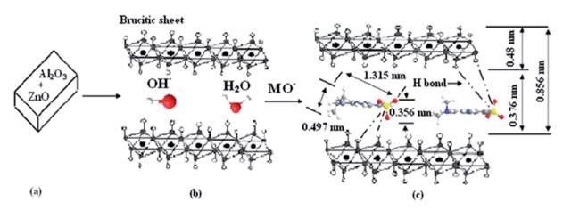
Fig. 12 The schematic illustration of MO adsorption by  $Zn-Al\ LDO$ . (a) The calcined layered double hydroxides. (b) The layered structure of recovered products is restructured by adsorption. (c) MO intercalated into LDH layered by chemisorption (adapted from ref. 88 with copyright from 2007 Elsevier).
