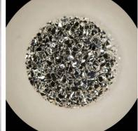
Fig. 3 Sublimate disk of magnesium (approx. 8 mm in diameter). Left: after removal from the lid. Right: microscopic image.
