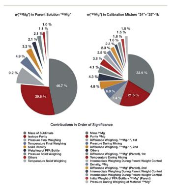
Fig. 6 Uncertainty budgets for the mass fraction of " $^{24}$ Mg" in the parent solutions " $^{24}$ Mg" (left), and in the binary calibration mixture " $^{24}$ " + " $^{25}$ "- $^{16}$  (right side).
