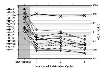
Fig. 5 Purification as a function of the number of sublimation cycles. All sublimations at 520 °C at the reference point.
