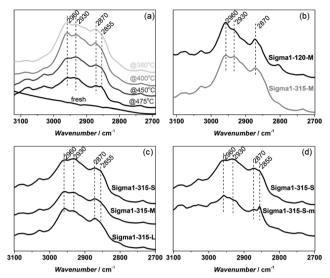
Fig. 12 DRIFT spectra of spent Sigma1-315-S catalyst used at different temperatures (a); Sigma1-120-M and Sigma1-315-M at 450 °C (b); Sigma1-315-S, Sigma1-315-M and Sigma1-315-L at 450 °C (c); Sigma1-315-S and desilicated Sigma1-315-S-m at 450 °C (d).
