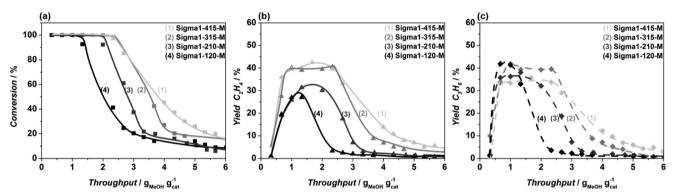
Fig. 6 Methanol conversion (a), yield of ethylene (b) and propylene at 450 °C, obtained in MTO reaction over Sigma1-415-M (III, A, ...), Sigma1-315-M (■, ♠, ♦), Sigma1-210-M (■, ♠, ♦), and Sigma1-120-M (■, ♠, ♦) zeolite at standard operation conditions.
