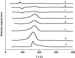
Fig. 5 TPR profile of (a) 5% Ru/TiO<sub>2</sub>, (b) 4% Ru-1% Pd/TiO<sub>2</sub>, (c) 3% Ru-2% Pd/TiO<sub>2</sub>, (d) 2.5% Ru-2.5% Pd/TiO<sub>2</sub>, (e) 2% Ru-3% Pd/TiO<sub>2</sub>, (f) 1% Ru-4% Pd/TiO<sub>2</sub>, (g) 0.5% Ru-4.5% Pd/TiO<sub>2</sub>, (h) 5% Pd/TiO<sub>2</sub>.
