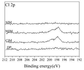
Fig. 3 Au(4f) and Cl(2p) spectra for 1% Au/TiO<sub>2</sub> samples prepared by different methods
