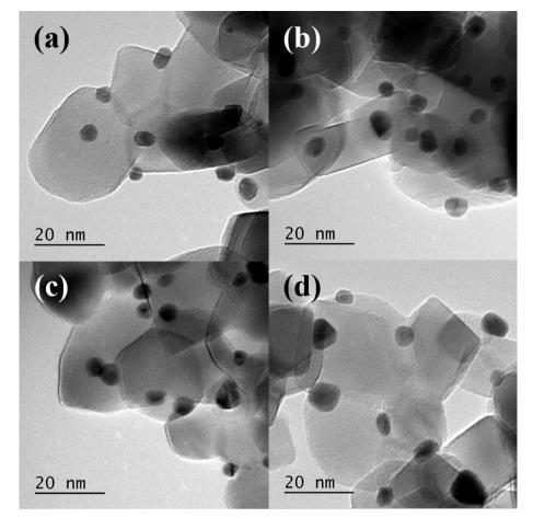
Fig. 6 Representative TEM images of 1% Au/TiO $_2$  SIM calcined at a) 250 °C, b) 350 °C, c) 450 °C and d) 550 °C.
