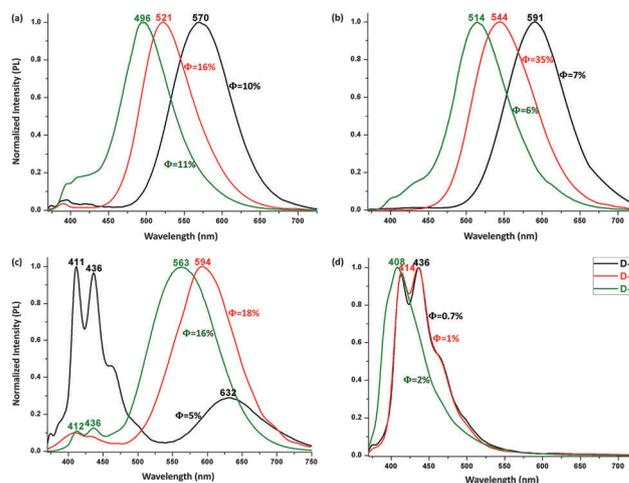
Fig. 3 Normalized PL spectra of **D-1**, **D-2** and **D-3** (2  $\mu$ M) in *c*-C<sub>6</sub>H<sub>12</sub> (a), CCl<sub>4</sub> (b), toluene (c) and CHCl<sub>3</sub> (d), with excitation at 350 nm.
