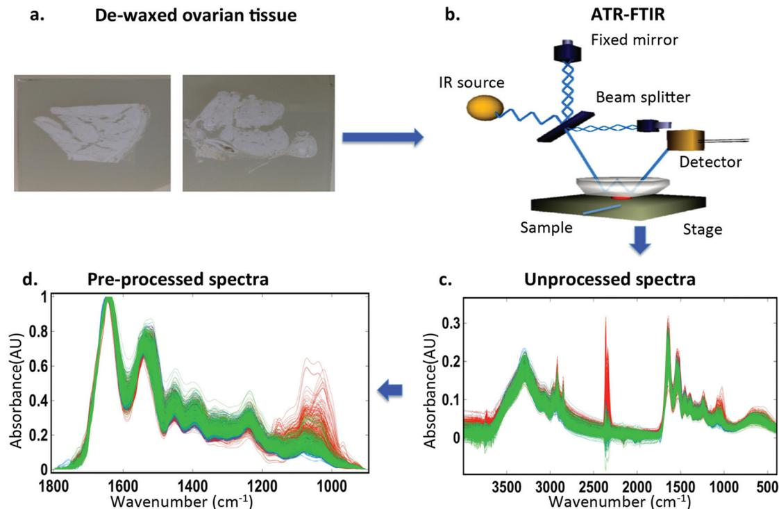
Fig. 2 Analysing ovarian tissues by ATR-FTIR spectroscopy and pre-processing resulting datasets. (a) 10  $\mu\text{m}$ -thick ovarian tissue sections; (b) sample in close proximity with the ATR diamond; (c) unprocessed spectra; and (d) resulting spectra after pre-processing.
