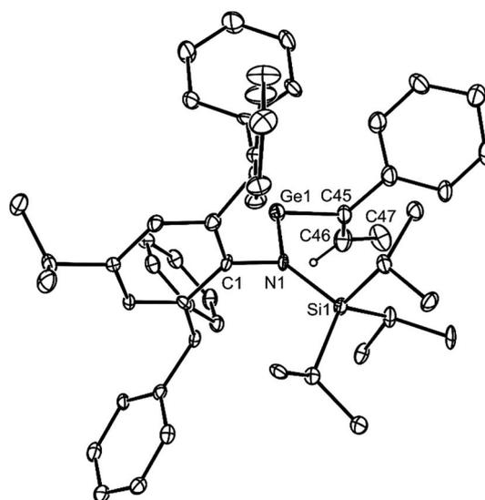
Fig. 2 Molecular structure of **14** (25% thermal ellipsoids are shown; hydrogen atoms, except the alkenic proton, omitted). Selected bond lengths (Å) and angles (°) for **14**: Ge(1)–N(1) 1.881(6), Ge(1)–C(45) 1.99(1), C(45)–C(46) 1.35(1), closest Ge(1)...C<sub>phenyl</sub> 3.27(1), N(1)–Ge(1)–C(45) 110.3(3). Selected bond lengths (Å) and angles (°) for **15**: Sn(1)–N(1) 2.122(5), Sn(1)–C(45) 2.229(8), C(45)–C(46) 1.32(1), closest Sn(1)...C<sub>phenyl</sub> 3.26(1), N(1)–Sn(1)–C(45) 107.1(2).
