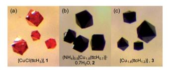
Fig. 2 Photos of (a) 1 CuCl(ttcH $_3$ ) crystals, (b) 2 – *i.e.* 1 treated in aqueous ammonia for 2 days, and (c) 3 – *i.e.* 2 dried at 130 °C under vacuum. The large monoliths are about 100  $\mu$ m across.
