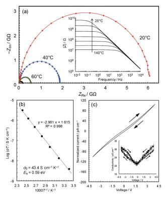
Fig. 3 AC impedance analyses. (a) Complex-plane impedance data for a pellet of 3 (red: 20 °C; blue: 40 °C; green: 60 °C; and black: 80 °C). The inset shows  $\log |Z|$  vs. log frequency plots. (b) Arrhenius plot of the electronic conductivity. (c) Current–voltage characteristics measured by cyclic voltammetry scanned at 10 mV s<sup>-1</sup> at 25 °C.
