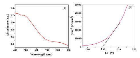
Fig. 3 (a) Diffuse reflectance spectra and (b)  $(\alpha h \nu)^2 vs. h \nu$  plot of ZnFe<sub>2</sub>O<sub>4</sub> annealed at 400 °C.
