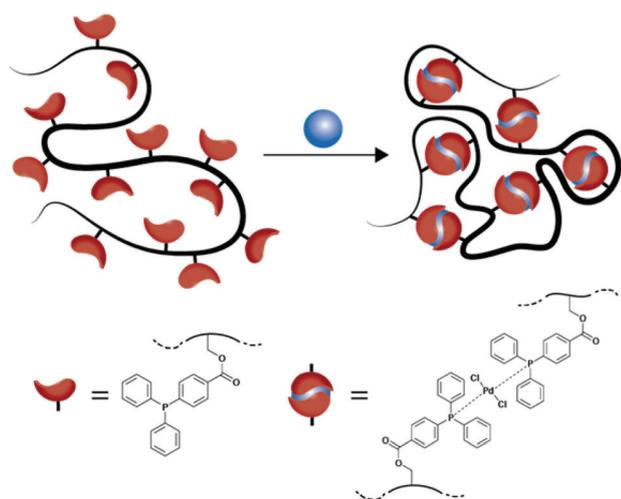
**Scheme 1** Illustration of the Pd-SCNP formation *via* the intramolecular crosslinking of functional, linear precursor copolymers by metal–ligand complexation in diluted solution (schematic view, in which we suggest a *trans*-configuration of the Pd-atoms, see text).
