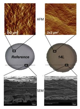
Fig. 4 AFM amplitude error images of  $4 \mu m^2$  areas of nanopaper surfaces (at the top) and SEM images of the cross-sections (at the bottom) of the reference and 14L samples.
