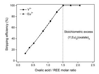
Fig. 10 Stripping of yttrium and europium from [Hbet][Tf<sub>2</sub>N] using pure (solid) oxalic acid. The influence of oxalic acid concentration on the stripping efficiency is shown. A ratio of 1.5:1 is the stoichiometric amount of oxalic acid required to precipitate all rare-earth ions (REE = Y + Eu) in solution as  $(Y,Eu)_2(C_2O_4)_3$  and results in a stripping efficiency of 10.0%
