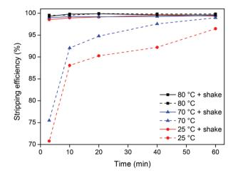
Fig. 9 Stripping kinetics and the influence of shaking (1500 rpm) are shown for 25 °C, 70 °C and 80 °C with 1 M HCl. The cloud point temperature is 74 °C and so at 80 °C the system is one homogeneous phase which explains the efficient stripping without shaking. For 25 °C and 70 °C it consists of two phases, a water phase and an ionic liquid phase, making shaking essential for an efficient stripping process.
