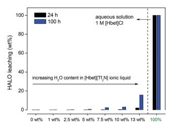
Fig. 3 Leaching (wt%) of HALO by [Hbet][Tf<sub>2</sub>N] at 90 °C (600 rpm) after 24 h and 100 h with increasing amounts of water in the ionic liquid: 0, 1, 2.5, 5, 7.5, 10 and 13 wt% (= water-saturated). Leaching is also shown in an aqueous solution containing [Hbet]Cl (1 M) which has a p $K_a$  of 1.83. <sup>43</sup>
