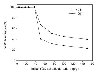
Fig. 6 Dissolution (wt%) of YOX in [Hbet][ $Tf_2N$ ] (5 wt%  $H_2O$ ) as a function of the initial YOX concentration in the ionic liquid (solid/liquid ratio). The dissolutions were carried out at 90 °C for 40 h and 100 h.
