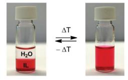
Fig. 8 Reversible formation of a homogeneous phase when increasing the temperature above the cloud point (55 °C for a pure water/ionic liquid system in a 1:1 ratio).44 A coloring agent (methyl red sodium salt) was dissolved in the transparent ionic liquid phase to help the visualization. The density of the [Hbet][Tf<sub>2</sub>N] liquid is higher than that of water.
