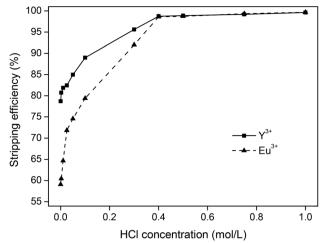
Fig. 7 Stripping of Y<sup>3+</sup> and Eu<sup>3+</sup> from [Hbet][Tf<sub>2</sub>N], previously loaded with 10 mg g<sup>-1</sup> of YOX. The influence of the HCl concentration on the stripping efficiency for Y<sup>3+</sup> and Eu<sup>3+</sup> is shown. The biphasic system was shaken (1500 rpm) at 25 °C for 1 h.
