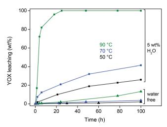
Fig. 4 Dissolution (wt%) of YOX in water-free [Hbet][ $Tf_2N$ ] and water-containing (5 wt%  $H_2O$ ) [Hbet][ $Tf_2N$ ] as a function of time and temperature.
