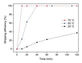
Fig. 11 Stripping of yttrium and europium from the [Hbet][ $Tf_2N$ ] ionic liquid, using a stoichiometric amount (3:2) of pure (solid) oxalic acid. The influence of time and temperature on the total stripping efficiency (Y + Eu) is shown.
