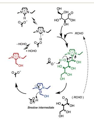
Fig. 8 Proposed scheme for condensation of [C<sub>2</sub>C<sub>1</sub>im][OAc], 1a, with open-chain D-(+)-glucose, 12, yielding the C1 adduct [C2C1(HO)C12im]+, 17 (red), via a Breslow intermediate (blue). The cleaved C(n-1) aldehyde fragment can react again with the parent ionic liquid, accounting for the intermediate adducts C5, C4, C3 and C2.
