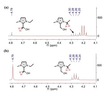
Fig. 6 (a) New <sup>1</sup>H NMR peaks (4.8–4.1 ppm) observed from the reaction of [C2C1im][OAc], 1a, with D-(+)-glucose, 12, after heating at 120 °C for 24 hours, assigned to the  $[C_2C_1(HO)C_1^2 im]^+$  cation. (b) <sup>1</sup>H NMR spectrum of synthesised  $[C_2C_1(HO)C_1^2im][OAc]$ , 17, for comparison.
