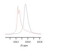
Fig. 6  $^{13}$ C NMR spectra showing the signal corresponding to the carbon at 2-position of [Bmim][CF<sub>3</sub>SO<sub>3</sub>] in either [Bmim][CF<sub>3</sub>SO<sub>3</sub>] (red) or [Bmim][CF<sub>3</sub>SO<sub>3</sub>] containing 4.5 wt% lignin (blue).
