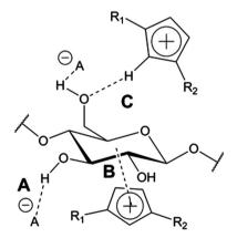
Fig. 5 Proposed dissolution mechanisms for cellulose in imidazolium-based ionic liquids: (A) interactions between the basic anion and the cellulose hydroxyl groups break up the hydrogen bond network between the cellulose chains. (B) Hydrophobic interactions take place between the hydrophobic face of cellulose and the imidazolium ring. (C) The acidic proton at the C-2 position on the imidazolium ring interacts with the cellulose hydroxyl groups.
