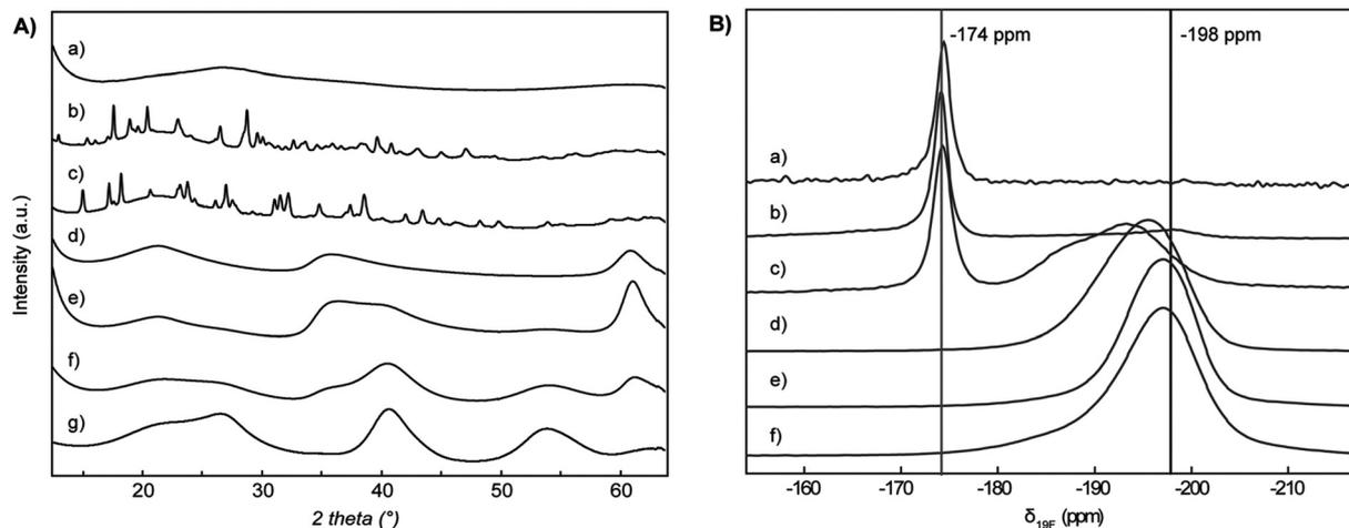
**Fig. 11** (A) X-ray powder diffraction patterns of  $\text{MgF}_x(\text{OCH}_3)_{2-x}$  with  $x = 0$  (a), 0.3 (b), 0.4 (c), 1 (d), 1.5 (e), 1.75 (f) and 2 (g), and (B)  $^{19}\text{F}$  MAS NMR spectra of  $\text{MgF}_x(\text{OCH}_3)_{2-x}$  with  $x = 0.1$  (a), 0.3 (b), 0.4 (c), 1 (d), 1.5 (e) and 1.75 (f); recorded in a 2.5 mm probe at 25 kHz. Reproduced from ref. 29b with permission of the Royal Society of Chemistry.
