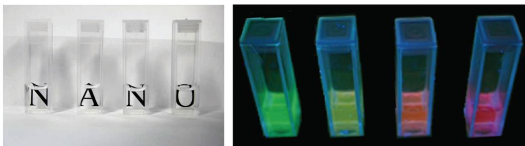
**Fig. 16** Picture of transparent  $\text{Eu}^{3+}$ - and  $\text{Tb}^{3+}$ -doped  $\text{CaF}_2$  sols (left) and the same sols excited with 366 nm (right). From left to right:  $\text{CaF}_2:\text{Tb}10$ , mixture of 52% of  $\text{CaF}_2:\text{Tb}10$  + 48% of  $\text{CaF}_2:\text{Eu}10$ ,  $\text{CaF}_2:\text{Tb}5.2,\text{Eu}4.8$  and  $\text{CaF}_2:\text{Eu}10$ ; reproduced from ref. 44 with permission of The Royal Society of Chemistry.
