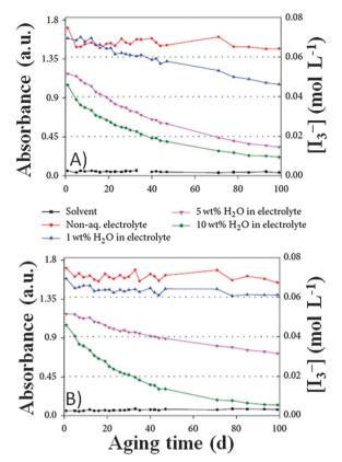
Fig. 22 Absorbance at 430 nm as a function of the aging time for DSSCs filled with solvent, non-aqueous electrolyte and redox electrolyte encompassing 1, 5 and 10 wt% H<sub>2</sub>O, in the presence of different GFs as sealants: (A) Bi<sub>2</sub>O<sub>3</sub>-SiO<sub>2</sub>-B<sub>2</sub>O<sub>3</sub>; (B) ZnO-SiO<sub>2</sub>-Al<sub>2</sub>O<sub>3</sub>. Adapted and reprinted from ref. 290.
