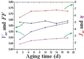
Fig. 20 Long-term stability under dark of DSSCs assembled with a fully aqueous electrolyte (KI 4.0 M and  $I_2$  20 mM at pH 8.0) and a PEDOT counter electrolyte. Dye: V35. PV parameters were measured under  $P_{\rm in}$  = 1 sun. Adapted and reprinted from ref. 249.
