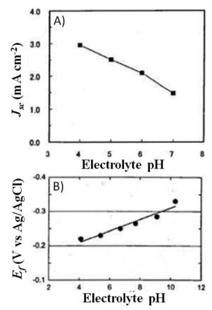
Fig. 18 (A) pH dependence of  $J_{sc}$  values ( $P_{in} = 1$  sun) obtained for an aqueous DSSC sensitized with N719. Electrolyte: KI 0.50 M and I<sub>2</sub> 25 mM; (B) dependence of the Fermi level electrochemical potential  $(E_f)$  of the mesoporous TiO<sub>2</sub> electrode on the pH of the above reported electrolyte. The potential data were based on the measurement of the onset potential of dark cathodic current. Adapted and reprinted from ref. 138.
