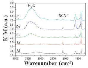
Fig. 5 DRIFT spectra of N719/TiO $_2$  films immersed in liquid electrolytes (LiI 0.50 M, I $_2$  50 mM and TBP 0.50 M in ACN) having different water contents for 192 h: (B) 0 vol% H $_2$ O; (C) 1 vol% H $_2$ O; (D) 2 vol% H $_2$ O; (E) 5 vol% H $_2$ O. The response of the photoelectrode before immersion is also shown (A) for comparison purposes. Adapted and reprinted from ref. 86.
