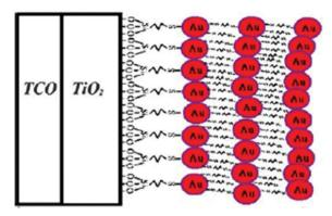
Fig. 15 Layer-by-layer Au NP assembly onto the TiO<sub>2</sub> electrode to act as a Schottky barrier in aqueous DSSCs. Adapted and reprinted from ref. 204.
