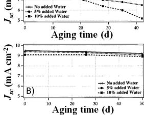
Fig. 17 Long-term stability ( $P_{in} = 0.015 \text{ mW cm}^{-2}$ ) of DSSCs assembled with RTIL-based electrolytes (I<sub>2</sub> 10 mM in HMII) encompassing different H<sub>2</sub>O contents. Dyes: (A) N3; (B) [Ru(H<sub>2</sub>dcbpy)(mhdbpy)(NCS)<sub>2</sub>]. Adapted and reprinted from ref. 231.
