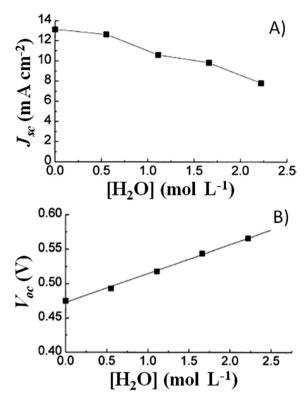
Fig. 3 Variation of  $J_{\rm sc}$  (A) and  $V_{\rm oc}$  (B) values, measured a 0.82 sun, due to water addition in the liquid electrolyte. Electrolytes: Lil 0.10 M and I<sub>2</sub> 10 mM in MAN/H<sub>2</sub>O. Dye: N3. Adapted and reprinted from ref. 43.
