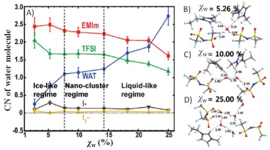
Fig. 23 (A) Dependence of water coordination (CN) on  $\chi_w$  in the presence of the following mole fractions: EMIm $^+$  0.50, TFSI $^-$  0.36, I $^-$  0.13 and I $_3$  $^-$  0.01. Representative water structure mediating EMIm+-TFSI- interactions after 30 ns molecular dynamics for: (B) ice regime, (C) nanocluster regime, and (D) liquid-like regime. Adapted and reprinted from ref. 299.
