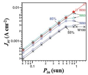
Fig. 9  $J_{sc}$  vs.  $P_{in}$  for selected water-free and water-based DSSCs (see Table 1). Percentages are  $J_{sc}$  relative to the water-free cell at the same  $P_{in}$  value. Adapted and reprinted from ref. 120.
