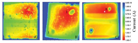
Fig. 6 Photocurrent maps for: (A) vacuum-filled ACN-based cell; (B) vacuum-filled aqueous cell; (C) high temperature vacuum-filled aqueous cell. The positions of the filling holes and the corresponding cold spots are indicated by the letters I-L. The side of each image is 1 cm. Adapted and reprinted from ref. 99
