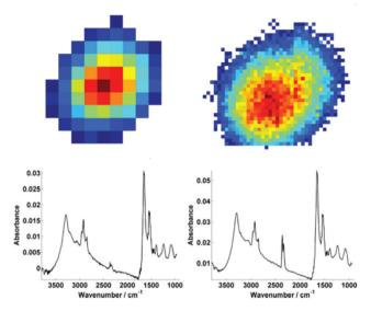
Fig. 3 An individual isolated single cell from the raw data chemimaps for both low (left) and high (right) magnification modes. For both modes, the respective mean spectra calculated from individual pixel spectra (63 spectra for low mag. and 905 spectra for high mag.) are shown below the respective map.
