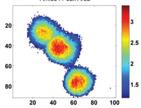
Fig. 4 (top-bottom) Photo-micrograph taken with a 40× objective, at a pixel resolution of 0.27  $\mu$ m. The amide I integrated peak area maps are presented for the raw spectral images acquired with normal and high magnification imaging modes respectively. The axes reflect the number of pixels, covering an area equivalent to  $\sim$ 100  $\times$  111  $\mu$ m.
