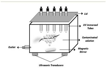
Fig. 6 Application of cavitation technology to photocatalysis by using ultrasonic transducers for efficient treatment of organic contaminants.
