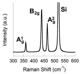
Fig. 2 Raman spectrum of few-layer phosphorene on a SiO<sub>2</sub>/Si substrate from liquid exfoliation of black phosphorus in NMP showing the characteristic Raman bands at 361 cm<sup>-1</sup>, 438 cm<sup>-1</sup> and 465 cm<sup>-1</sup> assigned to the  $A_g^1$ ,  $B_{2g}$  and  $A_g^2$  modes.
